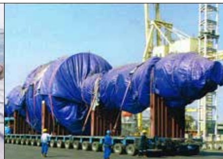
REACTOR Transportation (LxWxH @ 35.0X7.95X8.45 M)
