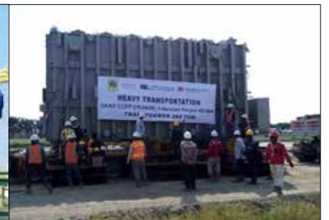
TRANSFORMER Transportation (LxWxH @ 11.8X4.4X5.5 M/288 TON)
