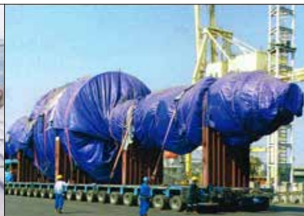
REACTOR Transportation (LxWxH @ 35.0X7.95X8.45 M)
