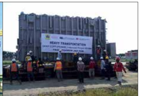
TRANSFORMER Transportation (LxWxH @ 11.8X4.4X5.5 M/288 TON)
