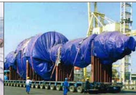
REACTOR Transportation (LxWxH @ 35.0X7.95X8.45 M)
