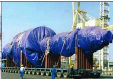
REACTOR Transportation (LxWxH @ 35.0X7.95X8.45 M)
