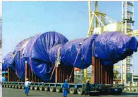
REACTOR Transportation (LxWxH @ 35.0X7.95X8.45 M)
