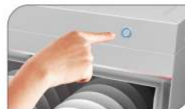
Start button for safety operation
